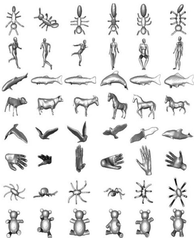
Fig. 9 Examples of shape retrieval with salient spectral geometric features. The 3D shapes at the left-most column are input queries, and those on the right are the first five retrieved results from the database
