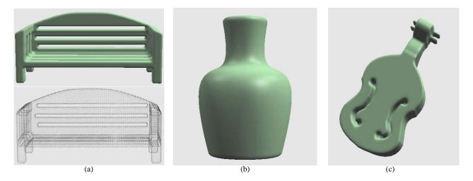
Figure 15: Some models from accurate point clouds. The sampling rates for these models are lower than the previous models. The Shepard's method works well for blending implicit fields generated at each sample point together. All the resulting models are rendered in polygonal meshes extracted by marching-cubes algorithm.
