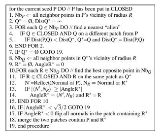
Table 2: Normal orientation alignment algorithm.
