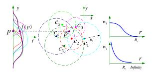
Figure 4: Shepard's local blending method. In the middle are a set of representative functions with their centers  $c_i$  and local support  $R_i$  marked. To the left are the projections of each weighted representative functions. To the right we show two classical weight functions.
