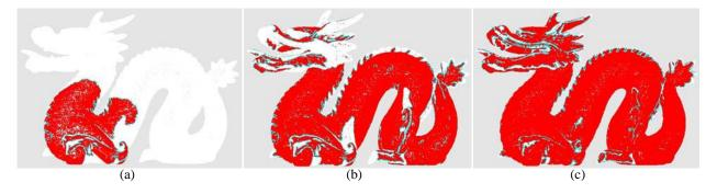
Figure 1: Prioritized incremental surface fitting. Red stands for the already fitted surface areas, green for the growing front and white for the untouched regions. The already fitted surface grows along an easier way, that is, along surface regions with smaller curvature and less noise.
